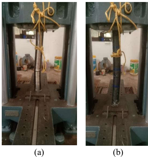
Fig. 3. Axial Compression Test on the Column: (a) unconfined LWCFST column and (b) CFRP-confined LWCFST column
