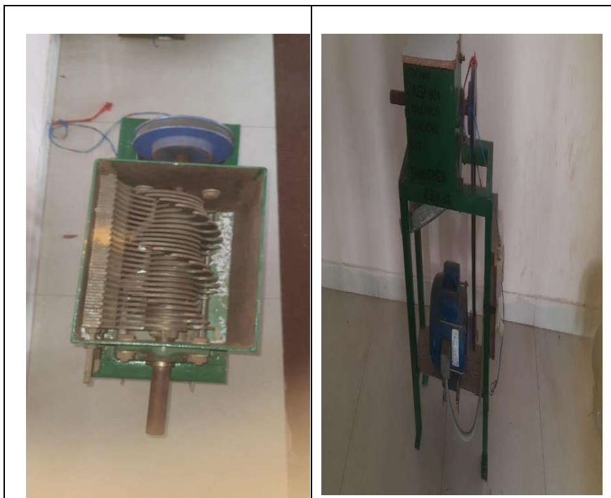
Figure 2: Sectional Views of Single-Shaft Shredder Machine
